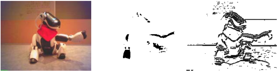
Fig. 2. Left: A robot pointing to its left side as seen from another robot's camera. The child robot tracks the adult robot in order to keep it in the centre of its visual field. Centre: Feature extraction for brightness using a threshold \theta . Right: Feature extraction for horizontal edges using a Sobel edge detector
