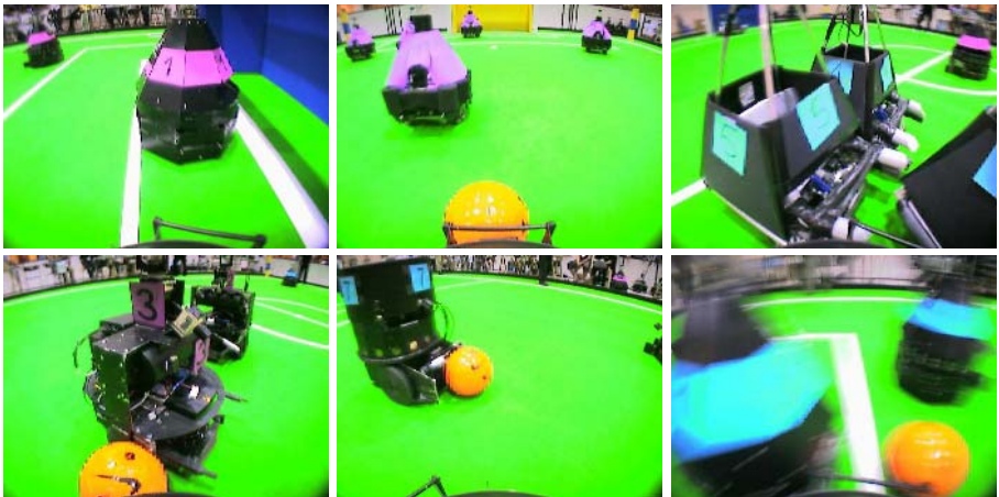
Fig. 1. Example images, taken from THE ULM SPARROWS, showing different types of perceptual difficulties. In the first two pictures (upper row) the variability in sizes of robots from the same type can be seen nicely. Recordings three and four showing occlusions, image five illustrates the lens distortion, which let the robot tilt to the left, and finally picture six is blurred by the robots own movement
