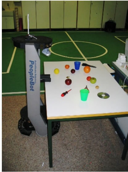
Fig. 4. In the test scenario the robot is situated in front of a table. Different objects are laying on this table. The robot has to grasp or point to specified objects
